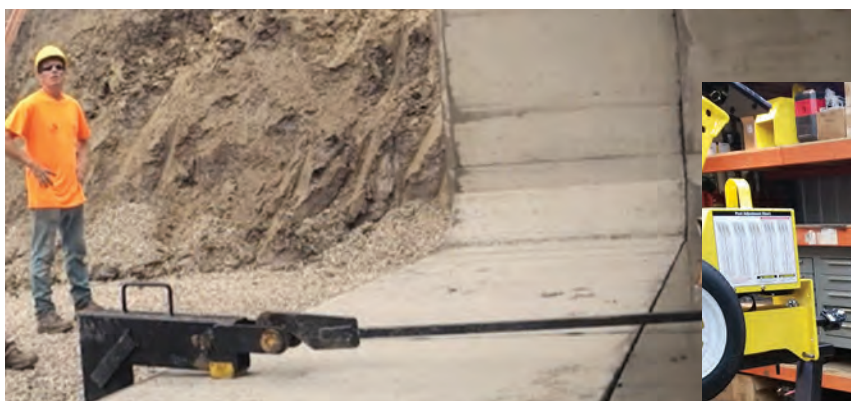
A J-Hook mounted on the side of a culvert.
